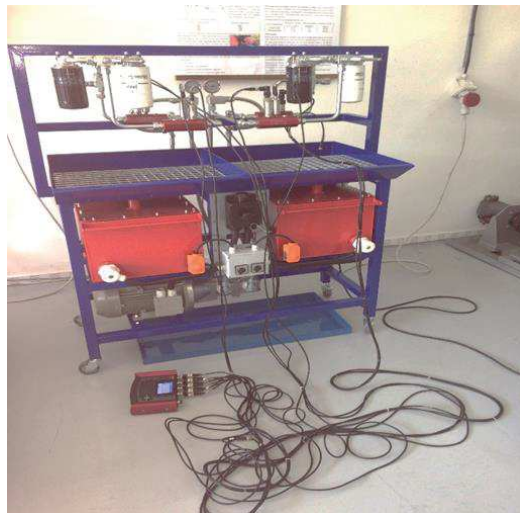
Fig. 3 Laboratory test equipment for comparing the flow properties of oil filter materials in the lubrication circuits of internal combustion engines
